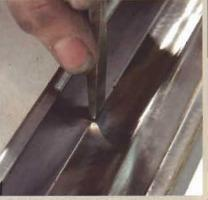
11 Using the rolled edge of a workbench as a dolly, the chisel end of a body hammer is used to work out the dent from the outside edge in toward the center.
