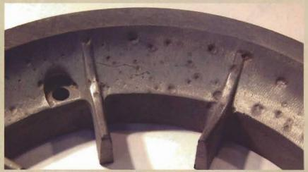
6 The only way to properly repair this taillight ring is to drill out each pit, fill each pit with silver solder, and then smooth each area before having it chromed. It's tedious work, but the shape of the part remains completely original.
