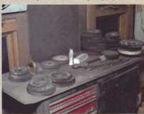
13 Using different buffing wheels for each compound is a must. If compounds are mixed on the wheels, smearing can result.
