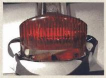
5 This taillight housing tooks great, but because the company that did the work fitted the pits by repeatedly copper plating it, the lens no longer fits in its opening. This method can work well, but because it causes parts to grow, care must be taken to remove excess copper build-up from critical fit areas.
