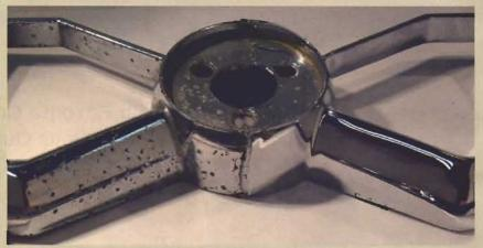
Half of this horn ring was done to show what's possible using the "drill and fill" method no wavy chrome on this one.
