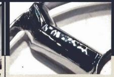
4 The pits on this pot-metal horn ring were ground smooth instead of being filled in. The pits are gone, but notice how wavy it looks after it was chromed. This part is ruined.
