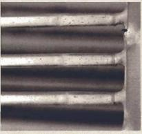
**2** Each of the little specks in this aluminum grill is a pit caused by corrosion that got through the anodizing. The only way to fix this is to remove the anodizing (already done here), and then gently sand each area smooth.
